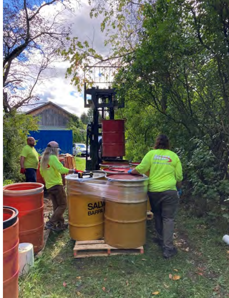
Contractors load compromised pesticide containers into overpack drums at an apple orchard
